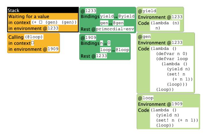
At this point, the oldest frame represents the top-level expression, which is waiting for the first call to gen to compute. Inside gen, we have initialized n to 0. Now we are about to start computing the (potentially) infinite loop.
