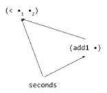
Suppose the value of seconds updates to become 10. This value is pushed, as we would expect, to *both* its *listeners*. This causes the (add1 seconds) node to update its value from 10 to 11. However, the update to seconds might have caused the comparison to occur immediately. At
